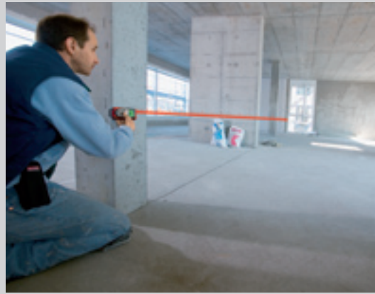
Room calculations: Pushbutton access to readings for room dimensions, wall and ceiling areas.
