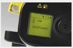
Tilt warning sensor -Keeps you on the level
