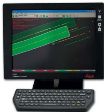
Airborne-qualified display with real-time coverage verification
