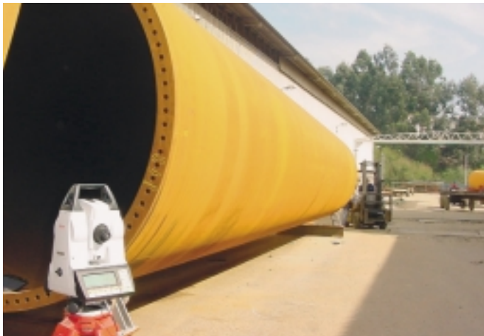
Component checking in wind-power stations at Tegopi in Portugal
