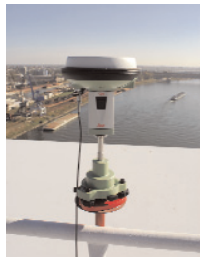
Leica Viva GS15 GNSS receiver on top of the bridge arch.
