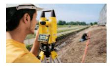
The Builder T100 or T200 can determine fill and drag points, define right angles and slopes.
