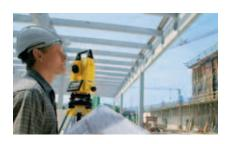
The Builder R100M and R200M with built-in memory, saves and transfers measured data via an interface between the Builder and a PC.
